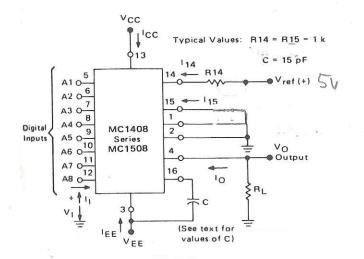
R14~ 3KJL RL~1KJL V<sub>1</sub> and I<sub>1</sub> apply to inputs A1 thru A8
