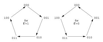
(i.e., when control line U=1 the circuit counts up to 4 (i.e., mod-5); when control line U=0 the circuit counts down from 4). Your job is to determine the gate arrangement needed to make this cycle run, i.e., connecting the outputs of the three JKFFs:  $Q_i$  (and/or  $\overline{Q}_i$ ) and the U line to the inputs of the three JKFFs:  $J_i K_i$  possibly using the usual (AND, OR,...) gates.
