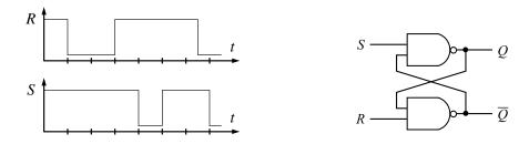
16. Consider the level-triggered active-high cross-NAND SR FF (HH Fig. 10.54) with S, R, CLK inputs (plotted as a function of time) as shown below. Graph Q (along with R, S, CLK) as functions of time.
