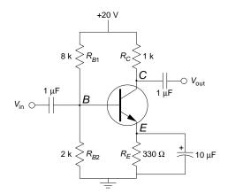
65. Design a BJT amplifier using the circuit shown right. You should provide all component values and the calculations that support those values. (This will require a choice for  $f_{-3\text{dB}}$ .) Calculate the input and output impedance. The circuit constraints are: voltage gain of 20, output impedance < 5 k $\Omega$ , input impedance > 15 k $\Omega$ , and that your base bias circuit will work for a transistor with  $\beta = 100$  or  $\beta = \infty$ .
