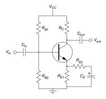
66. Design a BJT amplifier for a gain of 10 and an output impedance of 5 k $\Omega$  (i.e., find all the values for the components shown). Design the base bias assuming  $\beta=150$ . Assume the amplifier is to be used for audio frequencies in the range 20–20,000 Hz. Calculate the input impedance.
