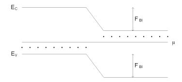
After equilibrium is established, there is balance between the diffusion current caused by the carrier inhomogenity (given by Ficks law) and the drift current caused by the electric field (given by simple kinetic free electron theory):
