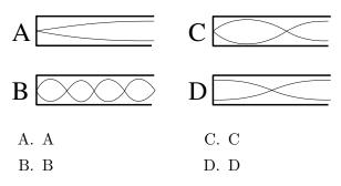
2. Which depicted standing wave (possible or impossible) shows a sound wave one octave above the fundamental of the open-closed organ pipe?
