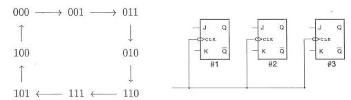
Your job is to design a synchronous circuit built from three edge-triggered JKFFs that follows the above state diagram, where the three binary digits  $Q_1Q_2Q_3$  are the outputs of distinct edge-triggered JKFFs. You will need to determine the gate arrangement needed to make this cycle run, i.e., connecting the outputs of the three JKFFs:  $Q_i$  to the inputs of the three JKFFs:  $J_iK_i$  possibly using the usual (AND, OR,...) gates.
