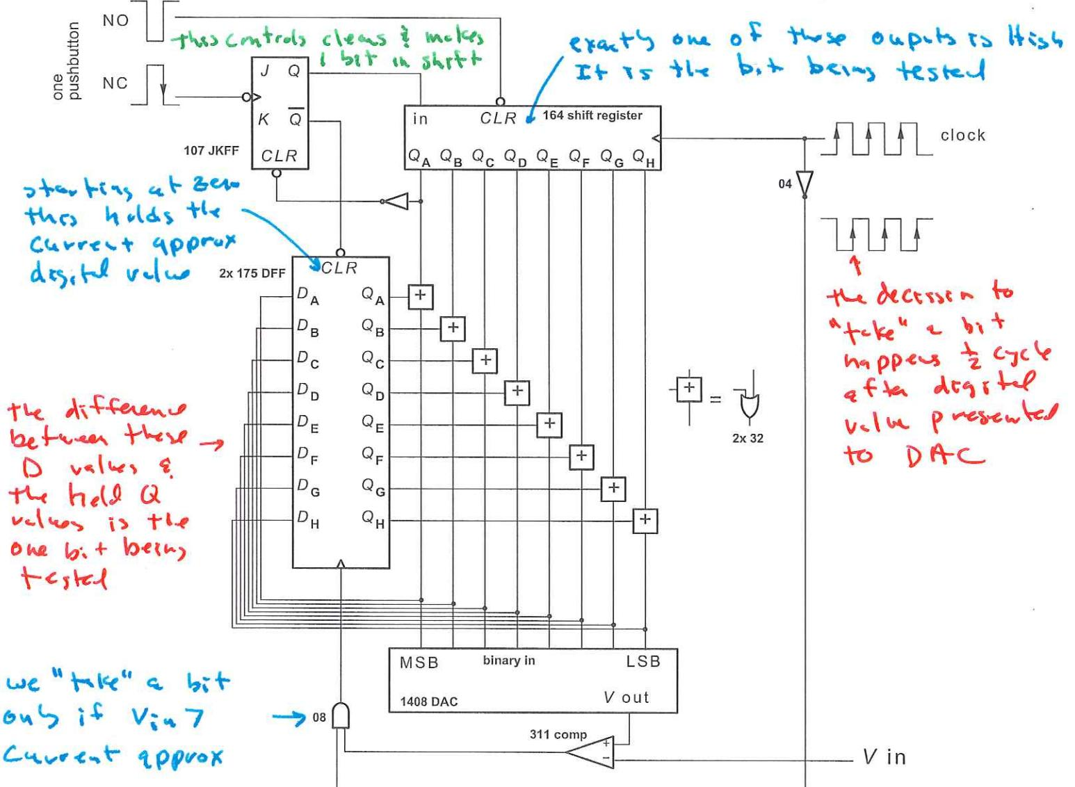
Note: in actual circuit 1408 DAC produces a negative voltage output. If thinking ab positive DAC outputs, reverse + - on compactor
