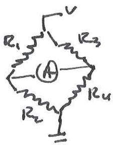
$$\text{if } \frac{R_1}{R_2} = \frac{R_3}{R_4} \text{ then } A = 0$$
