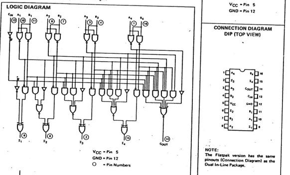
FUNCTIONAL DESCRIPTION - The LS83A adds two 4-bit binary words (A plus B) plus the incoming carry. The binary sum appears on the sum outputs ( $\Sigma_1 - \Sigma_4$ ) and outgoing carry (COUT) outputs.
