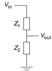
So if  $Z_2$  is a capacitor and  $Z_1$  is a resistor (i.e., our low pass filter) we have:
