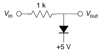
Extra Credit: The Thévenin equivalent circuit for the voltage divider circuit is a perfect voltage source in series with  $R_T$ . Construct this equivalent circuit (using the protoboard's +5 V supply as the perfect voltage source) and show that it responds to the diode clamp exactly as the voltage divider did. Note that you are seeing the reverse of 'voltage droop': here current goes in and as a result the voltage goes up.
