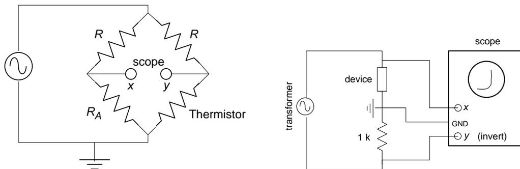
2. Diode Curve Tracer: “ $xy$ ” mode
