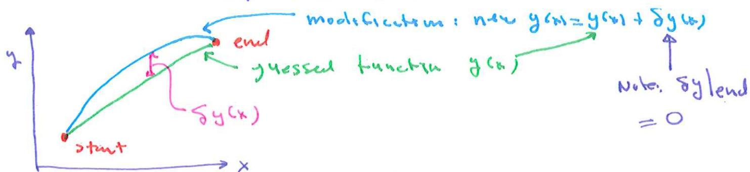
$$f(y + \delta y, y' + \delta y', x) \approx f(y, y', x) + \frac{\partial f}{\partial y} \delta y + \frac{\partial f}{\partial y'} \delta y'$$
