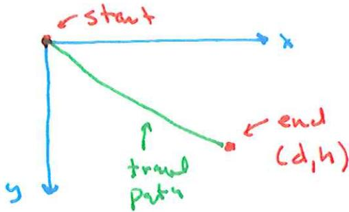
For this falling object the speed can be determined by conservation of energy
