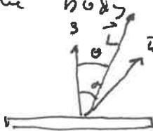
$$\tan\theta = \frac{\omega_1}{\omega_3} = \frac{I_1 \omega_1}{I_3 \omega_3} = \frac{I_1}{I_3} \tan\alpha = \frac{1}{2} \tan\alpha$$
