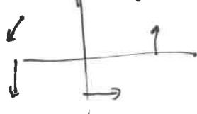
$$\begin{vmatrix} i & j & k \\ \frac{\partial}{\partial x} & \frac{\partial}{\partial y} & \frac{\partial}{\partial z} \\ -ky & kx & 0 \end{vmatrix} = \hat{i} \cdot 0 + \hat{j} \cdot 0 + \hat{k} \frac{2k}{r} \stackrel{\uparrow \text{ not zero}}{\phantom{=}} \stackrel{\text{not conserv}}{\phantom{=}}$$
