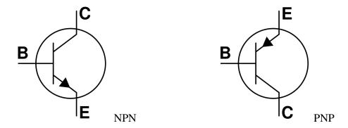
Bipolar Junction Transistor is a three terminals device with the Base, Emitter, and Collector electrode. Anyways, because of its fast respond and accuracy, transistor has been used in many applications such as amplifying or switching device.
