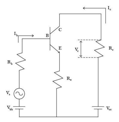
The diagram is a transistor amplifier circuit. The voltages  $V_{bb}$  and  $V_{cc}$  are fixed. To calculate the amplified signal  $V_s$  assuming there is a current gain,  $\beta$ , which means there current is  $I_c$ =  $\beta I_b$ , first is to apply the Kirchhoff's loop rule to the left hand loop, which will give:
